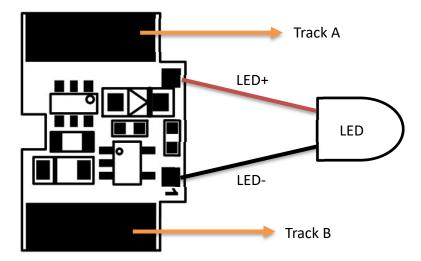
Connect the LED as shown in the figure. The red wire is connected to the positive terminal of the LED, and the black wire is connected to the negative terminal of the LED. The recommended size of the LED is SMD 0805 or SMD 0603.
