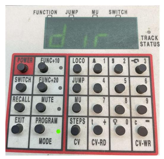
• Enter the CV address after pressing the CV key, and enter the write value after pressing the CV key once.
