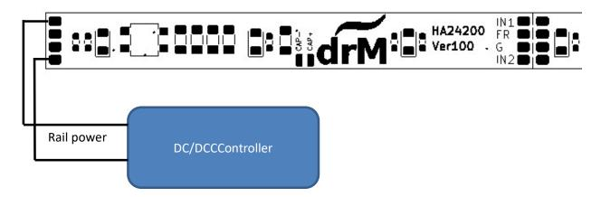
• IN1,IN2 of HA-24200 are power connecting ports. There is not polarity in this port. Please do not connect IN1 and IN2 to the same rail to prevent short circuit.
