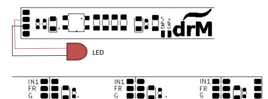
In the terminals of light bar, the ports which is marked with FR/G lables are reserved for Taillight. The FR is connected to anode of LED and G is connected to cathode of LED.
